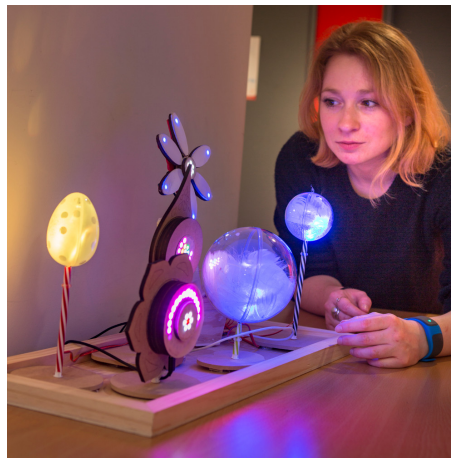
Figure 1: In this example heart-rate is measured through a smartwatch; tangible interfaces serve both as breathing guides for the user and as biofeedback devices (image © Inria, photograph C. Morel).
