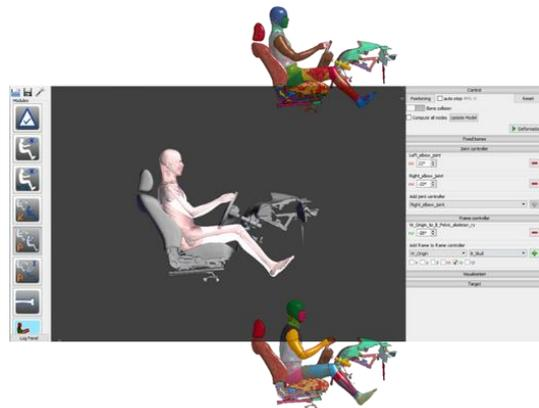
**Figure 3:** PIPER GUI with an example of FE model before and after positioning
