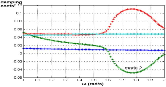
Fig. 2. Damping coefficients vs. blades angular velocity
