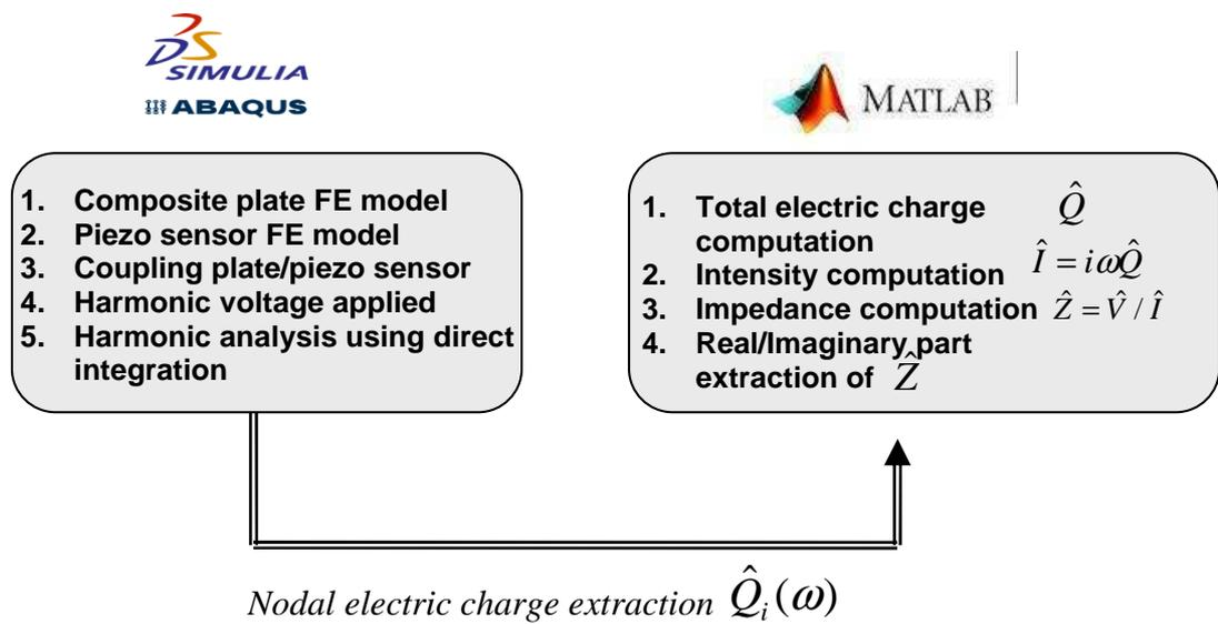
Figure 1: Modeling principle of the EMI technique.
