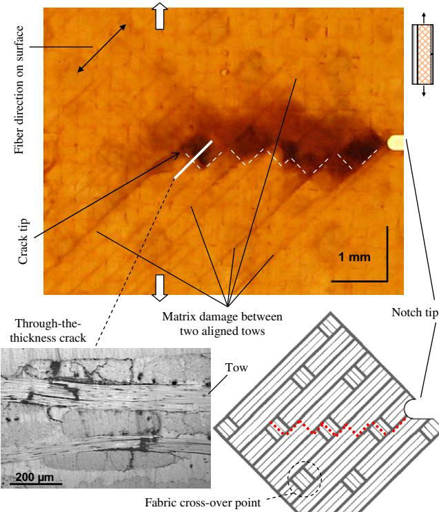
**Fig. 12.** Crack path in relation to woven fabric scheme in [45]<sub>2</sub> notched laminate loaded in fatigue.
