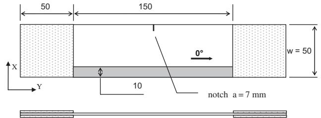
**Fig. 2.** Fatigue specimen test characteristics.
