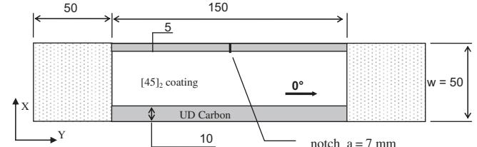
**Fig. 9.** Fatigue specimen test characteristics modified for  $[45]_2$  laminates.
