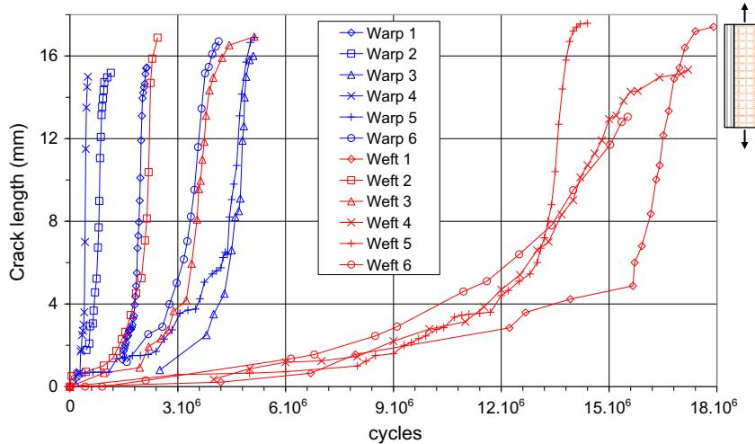
**Fig. 4.** Fatigue crack growth in warp [0]<sub>2</sub> (a) and weft [90]<sub>2</sub> (b) laminates in samples of 30 mm width.
