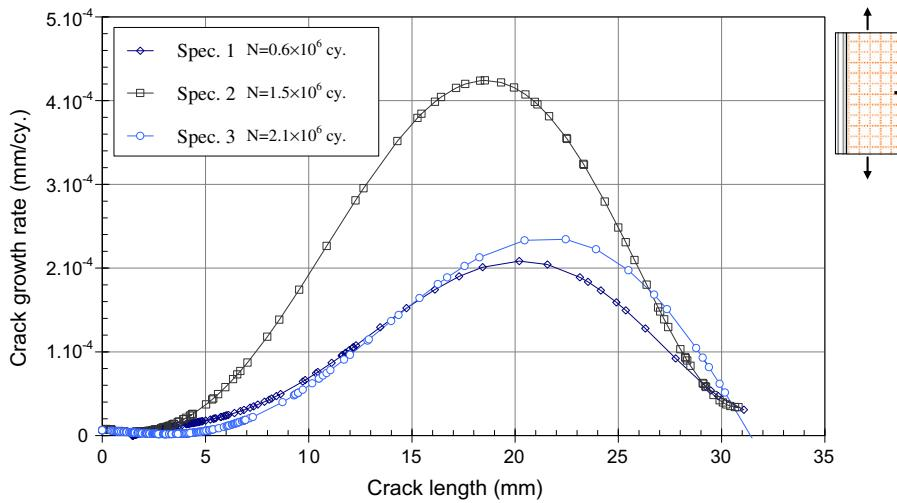
**Fig. 13.** Fatigue crack growth rate in [45; 0; 45] laminates.
