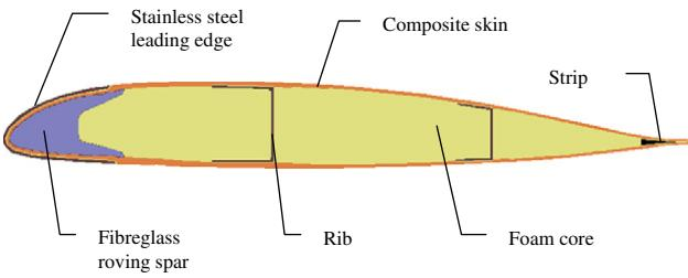
**Fig. 1.** Typical helicopter blade section.
