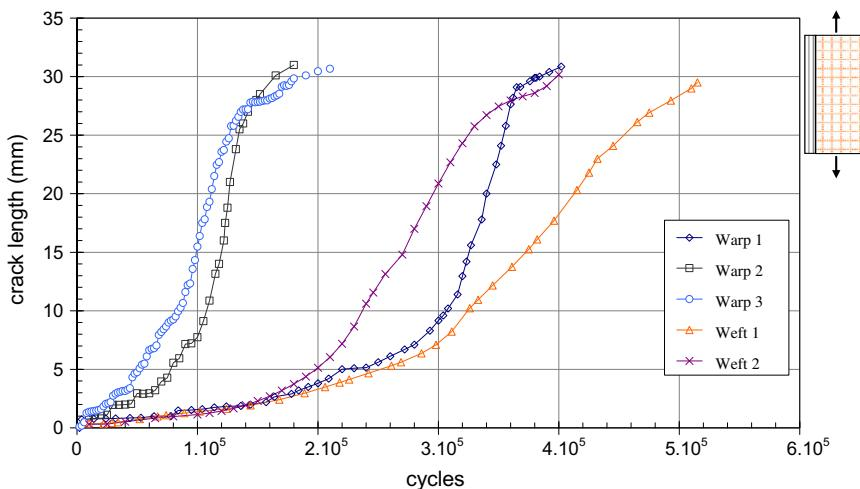
**Fig. 5.** Fatigue crack growth in warp [0]<sub>2</sub> and weft [90]<sub>2</sub> laminates in samples of 50 mm width.
