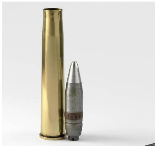
Fig. 5 Cartridge case and shell of a 40-mm Bofors gun.
