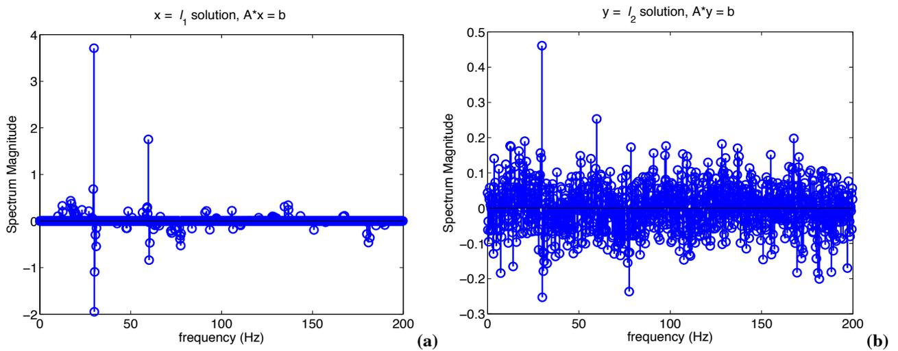
**Fig. 3. Comparison of DCT spectrum of reconstructed signals by  $\ell_1$  inversion (a) and  $\ell_2$  inversion (b) of randomized signals. The  $\ell_2$  inversion is not capable of good reconstruction (noise)**
