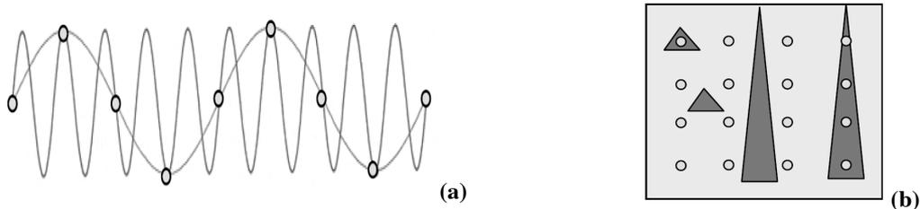
**Fig. 5.: In general artefacts are due to under-sampling or poor reconstruction: Temporal aliasing (Shannon's theorem) (a), Spatial aliasing (b) due to limited spatial resolution and induce loss of details.**
