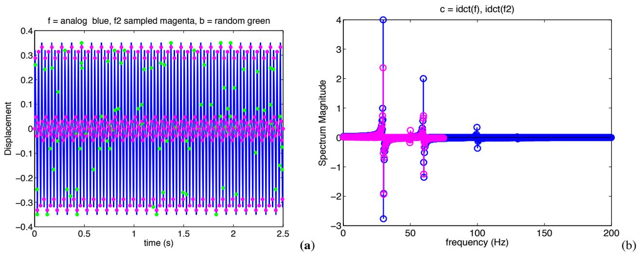
**Fig. 2. Analog signal (in blue), discretized signal (magenta) respecting Nyquist frequency (N points) and randomized signals at low resolution (N/10) (a), and DCT spectrum comparison (b)**
