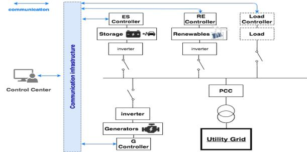
Fig. 1: Basic structure of a microgrid
