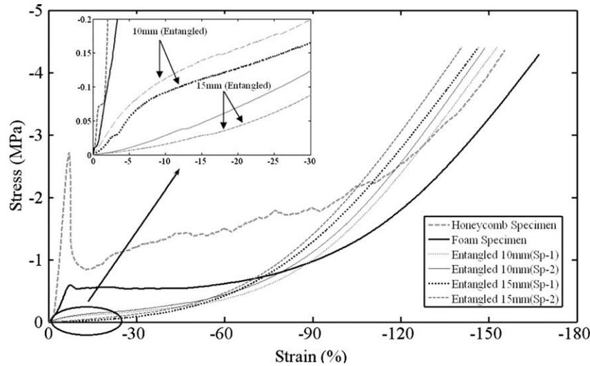
Fig. 7. Compression stress/strain curves for the entangled (10 and 15 mm fiber core length), foam and honeycomb sandwich specimens. The zoomed view shows the linear-elastic phase used for calculating the elastic modulus.
