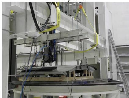
Figure 7: Impact test of the door
