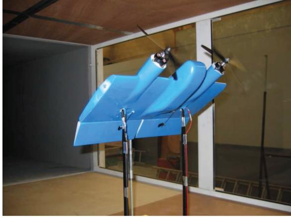
Figure 1: Wind tunnel model of MAVion.
