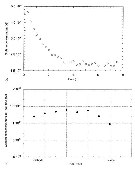
Fig. 4. Experiment without electric field: verification of the convective transport absence in soil. (a) Evolution of the sodium concentration at the cathode with time. (b) Sodium concentration into the soil after 7 h of experiment.
