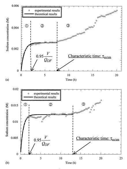
Fig. 5. Evolution with time of sodium concentration at the cathode: ( $\bigcirc$ ) experimental results; ( $\_$ ) simulation for  $t < \tau_{eo/em}$ . (a) Experiment A; (b) Experiment B.
