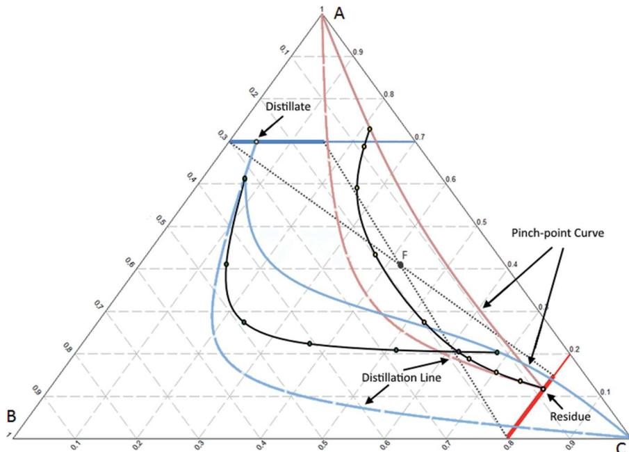
Figure 2. Theoretical number of stages: 5 stages in the rectifying section, 3 stages in the stripping section and the feed plate at the intersection which makes a total of 9 stages plus one total condenser and one reboiler
