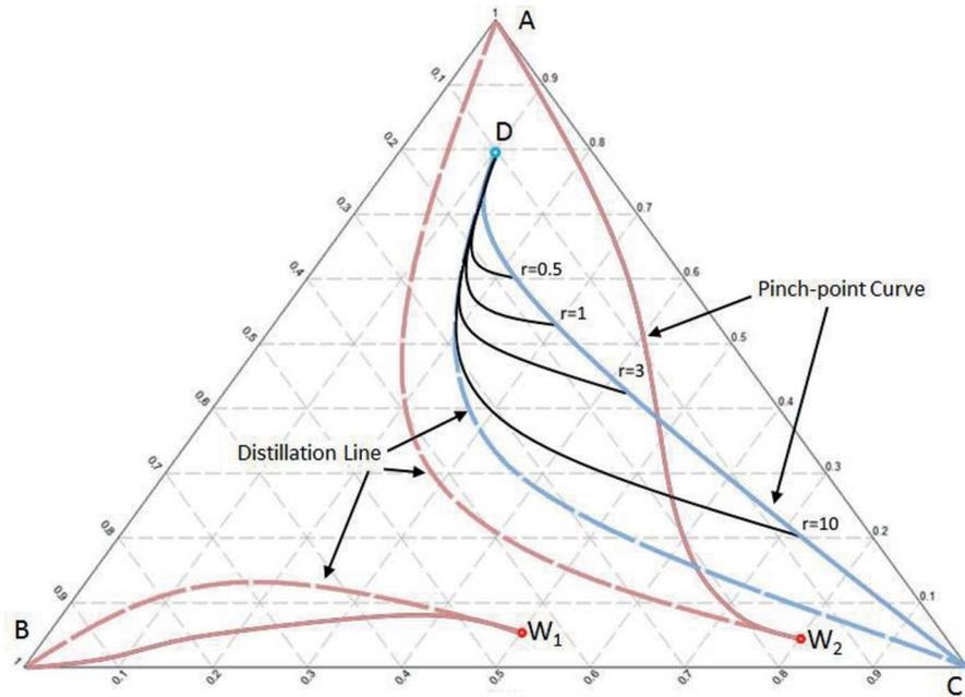
Figure 1. Operation leaves in a A (light), B and C (heavy) ternary diagram - Separation of D and W1 is unfeasible whereas separation of D and W2 is feasible. Operation leaf of D shows some liquid composition profiles for some values of the reflux ratio
