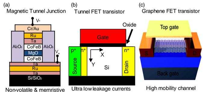
Figure 2. (a) a non-volatile and memristive nanodevice: magnetic tunnel junction composed of ferromagnetic and oxide thin films [6] (b) an ultra low  $I_{off}$  nanodevice: Si-channel based tunnel FET [14] (c) a nanodevice with high mobility channel: Graphene FEF transistor [7].
