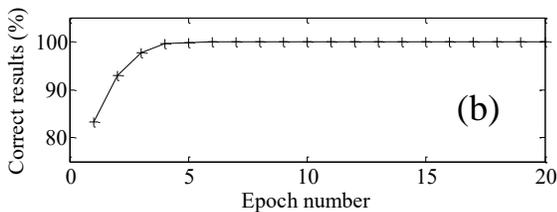
Figure 4. (a) Architecture of a “neural learning block” with a memristor crossbar array and CMOS neuron circuits. (b) Simulation of the system trained to learn the 104 linearly-separable digital functions with 3 inputs and 1 output. Proportion of correct answer of the network for successive presentation of a truth table (“epoch”). After 10 presentations, all the functions have been trained.
