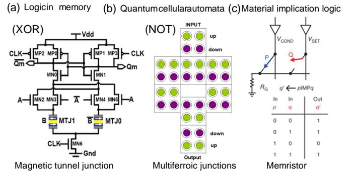
Figure 3. (a) Logic in memory architecture: XOR logic composed of magnetic tunnel junction memory cell [21] (b) Multiferroic cell based QCA NOT logic [12] (c) Memristor based IMP logic [13].
