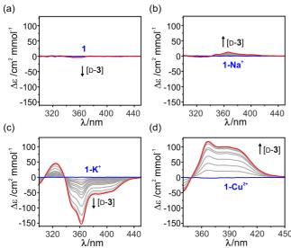
Fig. 2 Induced CD spectra upon binding of D-3 by: (a) 1, (b) 1-Na<sup>+</sup>; (c) 1-K<sup>+</sup>; (d) 1-Cu<sup>2+</sup> at 298 K, [host] =  $60 \mu M$ , 9:1 (vol/vol) CHCl<sub>3</sub>/DMSO. Red-coloured spectra in (a-d) denotes the molar ellipticity of the hosts in the presence of D-3 at the concentrations of 21, 19, 32 and 2 mM, respectively.
