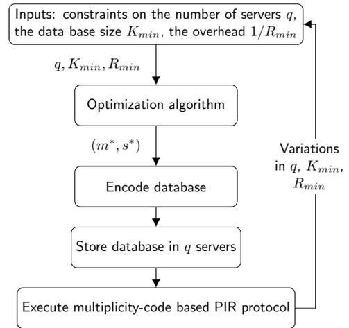
Fig. 1: Adaptive Multiplicity Codes Based PIR Protocol
