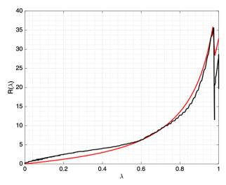
Fig. 34 Force (N) versus non-dimensional displacement for the shear test of a pantographic sheet up to the onset of fiber breakage. The black curve is the experimental data, and the red curve has been obtained via numerical simulation (color figure online)
