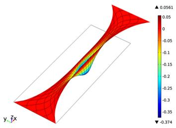
Fig. 23 Simulation of bias extension test on parabolic pantographic fabrics. Out-of-plane buckling is observed after a critical loading. Deformed configuration and qualitative out of plane displacement
