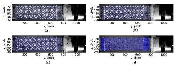
Fig. 39 Finite element meshes overlaid with the gray-level picture of the reference configuration
