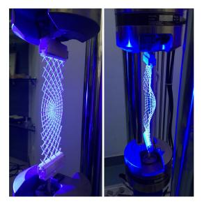
Fig. 22 Bias extension test on parabolic pantographic fabric. Out-of-plane buckling is observed after critical loading
