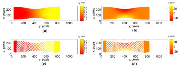
Fig. 41 Longitudinal (a-c) and transverse (b-d) displacement fields measured with meshes 3 (a, b) and 4 (c, d) for the 10th picture. The fields are shown on the deformed configuration
