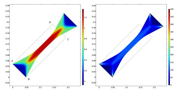
Fig. 15 Numerical simulation of the bias extension test. Colors indicate the shear strain relative to the initial fiber axes (left) and the strain energy density (right) [13]
