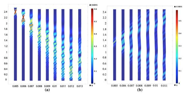
Fig. 29 Qualitative displacement plot of a wave propagating after a prescribed vertical displacement on the upper side (left). Wave propagating after double impulse (right)
