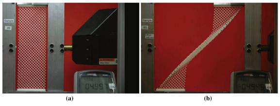
Fig. 32 a Reference configuration ( $\lambda = 0$ ), **b** damage onset ( $\lambda = 0.976$ ) of a shear test
