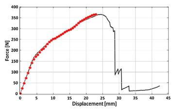
Fig. 36 Force versus applied displacement for a uniaxial bias extension test of an aluminum pantographic sheet. The black curve is the experimental measurement and the red obtained via numerical simulation (color figure online)
