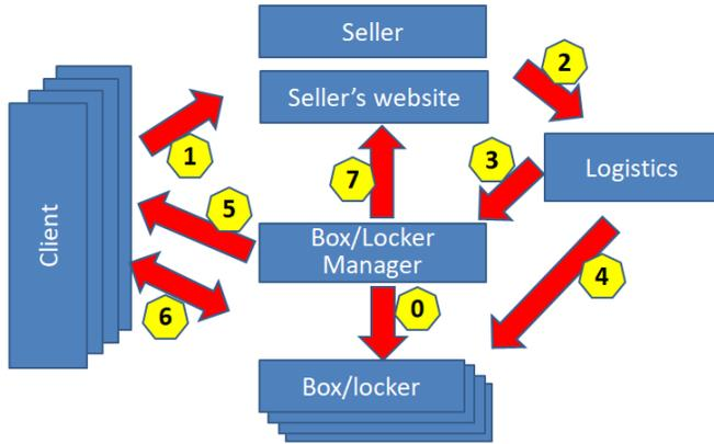
Fig. 2. Software architecture with main modules and exchanges.
