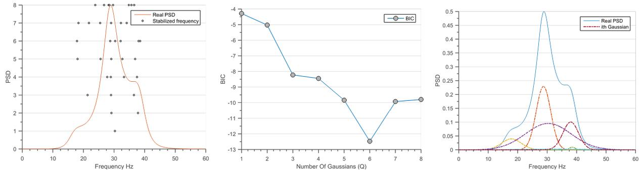
(a) Stabilization diagram with increasing number of gaussians  $Q$ , the dots denote the stabilized frequencies. We can observe that as the number of  $Q$  increases the algorithm starts finding better and better modes.
