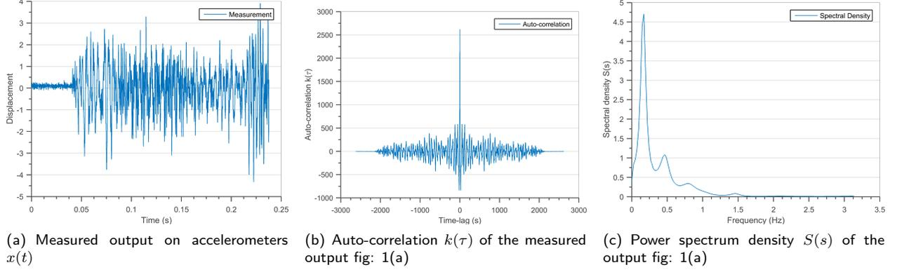
**Figure 1: Different types of measurements for estimation of Modal parameters in OMA**
