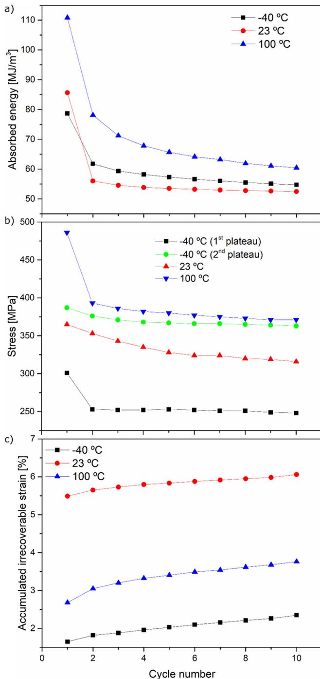
**Fig. 11.** a) Evolution of the accumulated irrecoverable strain with the number of load/unload cycling tests; b) Evolution of the stress onset for the forward martensitic transformation with the number of load/unload cycling tests; c) Evolution of the absorbed energy with the number of load/unload cycling tests.
