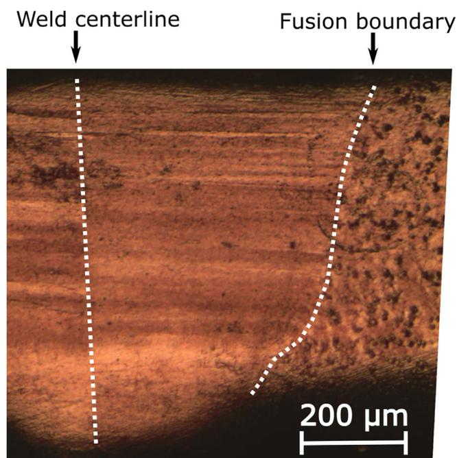
Fig. 2. Microstructure of Cu-Al-Be laser welded joint.
