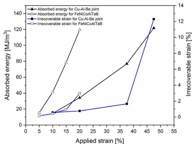
**Fig. 9.** Evolution of the absorbed energy and irrecoverable strain as a function of the applied strain during superelasticity cycling: comparison between the Cu-Al-Be laser welded joint and the Fe<sub>28</sub>Ni<sub>17</sub>Co<sub>11.5</sub>Al<sub>2.5</sub>Ta<sub>0.05</sub>B (at. %), noted as FeNiCoAlTaB, shape memory alloy [41].
