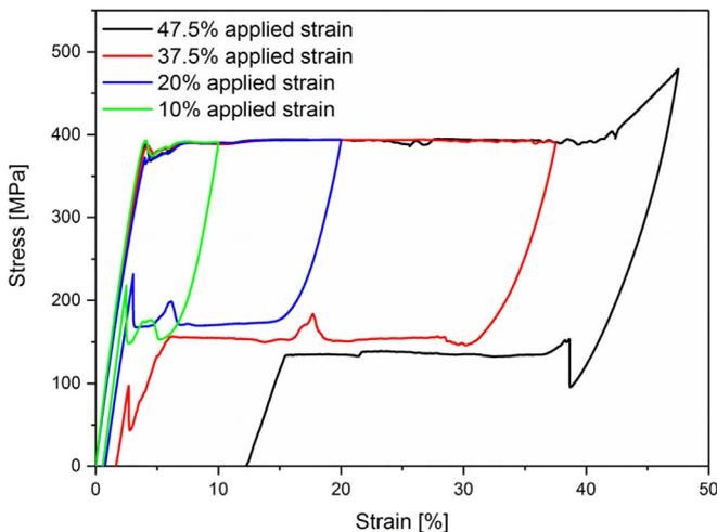
**Fig. 7.** Load/unload cycling behaviour of the welded joints.
