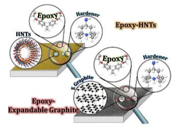
Fig. 2. Schematic of chemical structure of EG/epoxy and HNTs/epoxy composites.
