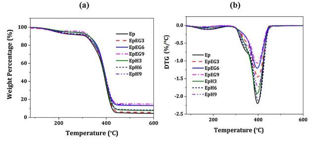
Fig. 4. (a) TGA and (b) DTG curves of all samples at heating rate of 10 °C.min-1 under nitrogen.
