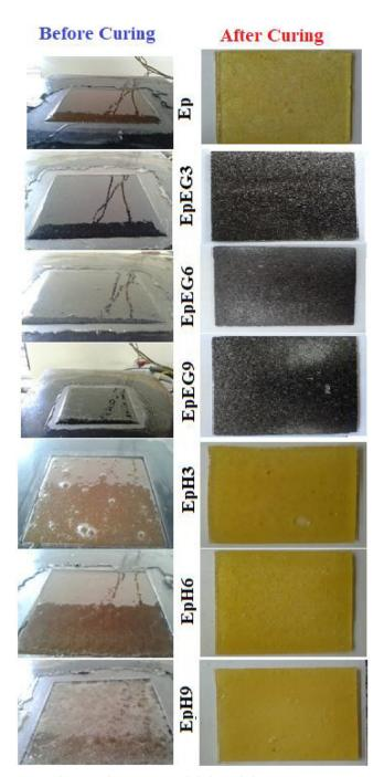
Fig. 3. Samples' appearance right before and after curing process.
