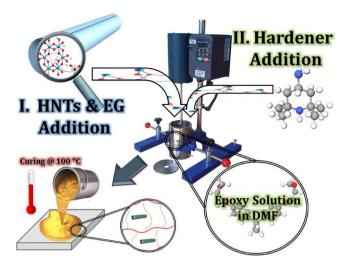
Fig. 1. Schematic of procedure applied in sample preparation.
