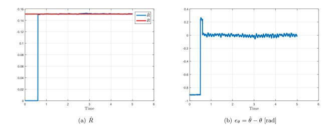
Figure 7: Real data: Results of the observer algorithm discussed in Section 5.2, with  $\lambda_1 = 40$ ,  $\lambda_2 = 50$ ,  $\lambda_3 = 60$ ,  $dt_R = 0.1$ , and a grid with amplitude G = 1. The estimation starts at t = 0.5.
