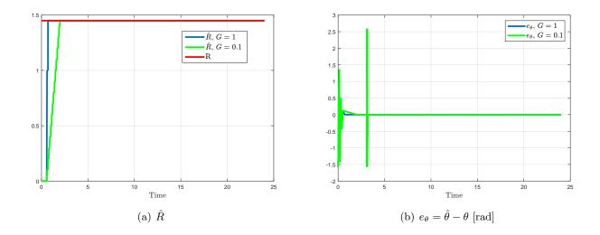
Figure 3: Ideal data: Results of the observer algorithm discussed in Section 4.1 with  $\lambda_1 = 20$ ,  $\lambda_2 = 30$ ,  $\lambda_3 = 40$ ,  $dt_R = 0.1$ , and two grids with amplitude G = 1 and G = 0.1 respectively. The estimation starts at  $\bar{t} = 0.5$ .
