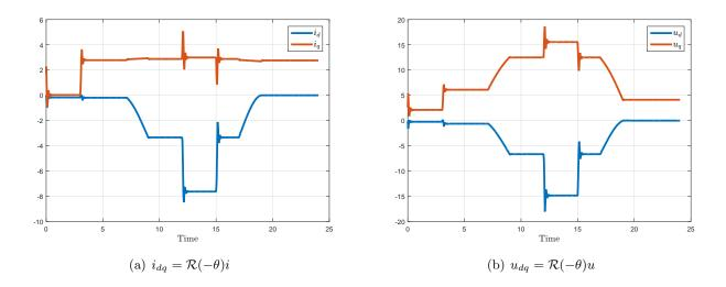
Figure 2: Ideal data: currents and voltages in the rotating frame.
