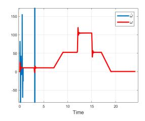
Figure 1: Ideal data: Rotation speed  $\omega = \dot{\theta}$  and estimated rotation speed  $\hat{\omega} = \hat{\theta}$ . The estimation algorithm starts at  $\bar{t} = 0.5$ .
