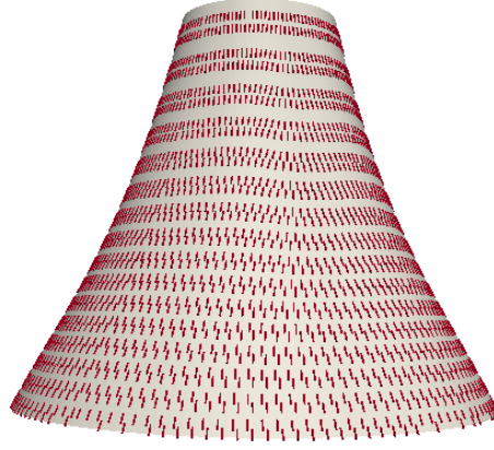
Figure 15: Example two, shape and anisotropy optimization: optimal shape and material orientation.
