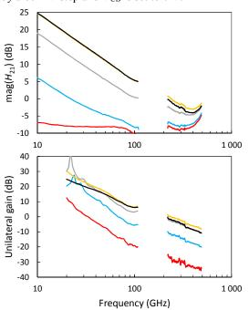
Fig. 6: Unilateral gain and Current gain H21 of a 2\*CBEBC SiGe HBT of  $(0.22*1\mu m^2)$  drawn emitter window size from Infineon for different  $V_{BE}$  ranging from 0.7-0.94 V with 60 mV step and  $V_{CB}$ =0 V, using an on-wafer TRL calibration with impedance correction, plus move of the reference plane above vias at M6 (see Fig. 2).
