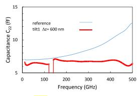
Fig. 9: Capacitance "C22" versus frequency of the transistor-open obtained from EM simulation including a TRL calibration with an ideal probe and with tilt default (reference: Δz=0nm, tilt1: Δz=600nm).
