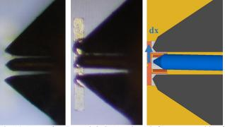
Fig. 14. Image of a 50 µm pitch CPW probe a) before contact and b) after contact on a used ISS short standard. The probe flexibility in combination with a deteriorated ISS standard causes a deformation of the probe eventually modifying its characteristic impedance; c) Geometrical Model for EM simulation showing a default on CPW probe (dx=6µm movement at port 2).
