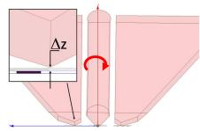
Fig. 8: EM model used for planarity of the probe (reference:  $\Delta z$ =0nm, tilt1:  $\Delta z$ =600nm contact is lost in the last case)
