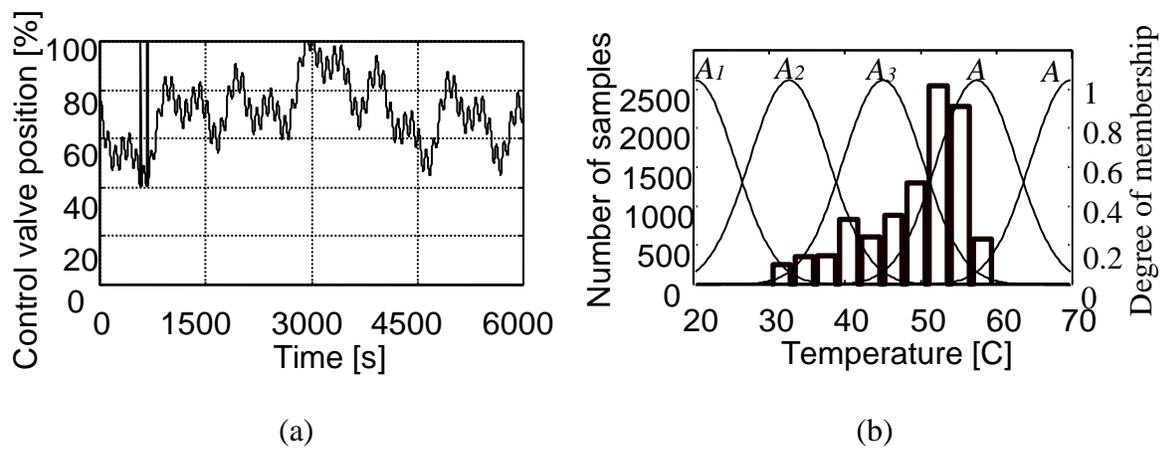
Figure 3 Characteristics of the signals used for identification: (a) time sequence of the input signal; (b) histogram of the output signal superimposed with the membership functions.
