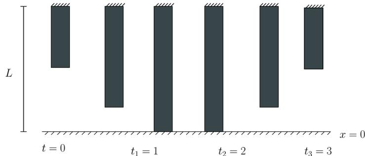
Figure 1: Multiple impacts of an elastic bar. The bar is clamped at  $x = L$  and the contact node is located at the bottom. The closed-form solution is periodic of period 3, with one impact during each period (here between  $t = 1$  and  $t = 2$ ).
