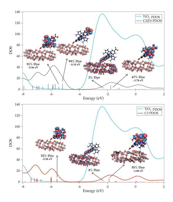
**Figure 4.** Projected DOS (PDOS) and main dye's MOs isodensity plots for the deprotonated **C2(D)** (top) and heteroleptic **C5** (bottom) complexes adsorbed onto the (TiO<sub>2</sub>)<sub>82</sub> cluster. For the depicted MOs the % contribution of population localized on the dye is also indicated. The gaussian broadening used to reproduce the PDOS is equal to 0.3 eV. Vertical sticks represent the Khon-Sham eigenvalues and their intensity the % dye's population.
