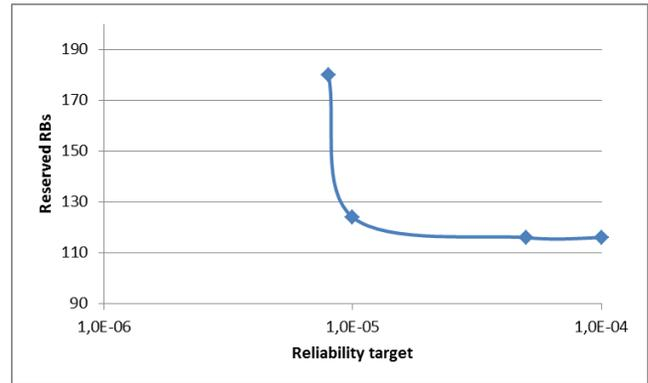
Fig. 4. Number of RBs to be reserved for different reliability targets for a mix of users with good and bad radio conditions.
