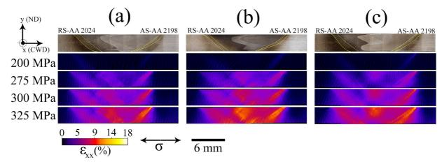
Fig. 12. Local in-plane strain distribution obtained with DIC for joints E1, F1 and G1. The strain localization for all tools are in TMAZ/HAZ of AA2198 and center of nugget.
