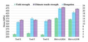
Fig. 11. Mechanical properties of FSW joints produced by tools E, F and G at  $750\,\mathrm{rpm}$  and  $50\,\mathrm{mm\,min}^{-1}$ . The joint produced with tool F demonstrated higher mechanical strength and elongation.
