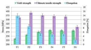
**Fig. 17.** Mechanical properties of FSW joints produced by tool F according to welding speed parameters in Table 3. Parameters 750 rpm and 450 mm min<sup>-1</sup> (sample F4) produced the joint with highest yield strength.
