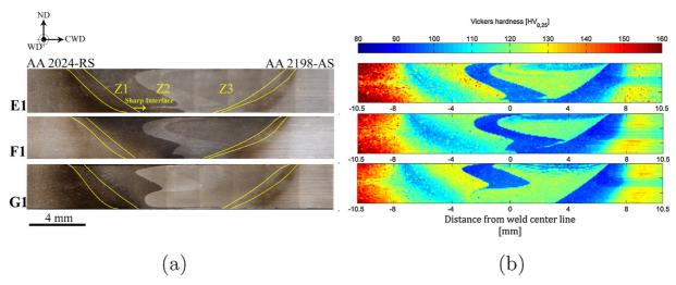
Fig. 6. Cross-section observations of samples E1, F1, and G1. (a) Nugget region delimited by yellow solid lines on CWD-ND cross-section where the different colors resulting from etching are denoted zones Z1, Z2, and Z3. (b) Corresponding 2D microhardness maps showing the minimal hardness values in Z2 zone, shoulder affected area, and TMAZ/HAZ on AA2198 side.
