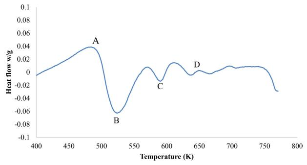
Fig. 10. DSC and temperature measurements, (a) DSC result of base metal AA2198-T3 and (b) temperature measurement of TMAZ on both joint sides.
