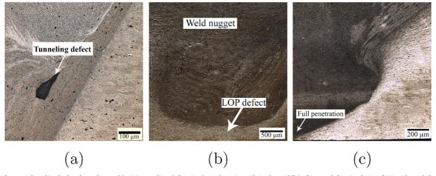
Fig. 5. Defects produced in the bead-on-plate welds: (a) tunneling defect (tool A, advancing side in the middle), (b) LOP defect (tool A) and (c) without defect (tool E, advancing side).
