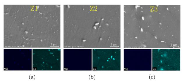
Fig. 9. SEM micrographs of Z1, Z2 and Z3 zones and the related EDS maps for elements Mg and Cu. (a) Zone Z1, (b) Zone Z2 and (c) Zone Z3. Zone Z1 has different precipitates in comparison with Zone Z2 and Z3.
