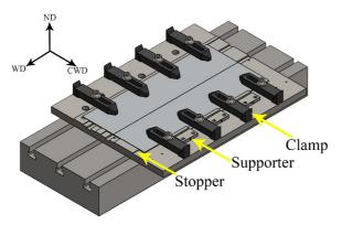
**Fig. 1.** Fixture designed for the repeatability of the FSWed joints. The welding plates are fixed by stoppers, supporters, and clamps in the directions WD, CWD, and ND respectively.
