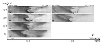
Fig. 15. Cross-sectional macrographs of joints produced by tool F with parameters of Table 3. The tunneling defect was found in only joint F6 with the highest rational speed (1000 rpm) and highest traverse speed (450 mm min<sup>-1</sup>).
