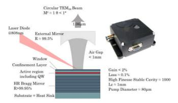
Fig. 1. VECSEL architecture, physical parameters, and packaging.
