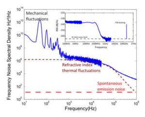
Fig. 6. Frequency noise spectral density and intensity noise spectral density (inset).
