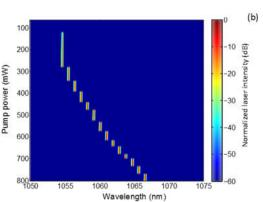
Fig. 3. Optical spectrum tunability of the VECSEL by setting different operation temperature at 600 mW of pump power (a) and the recorded emitting wavelength at various pump powers (b).
