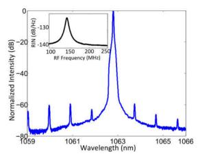
Fig. 5. Optical high-resolution spectrum at high output power and RF spectrum of the beating between the two polarization modes (inset).
