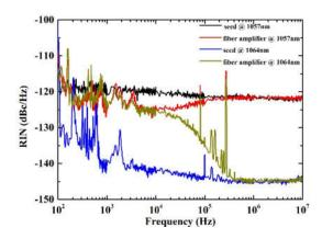
Fig. 8. Relative intensity noise measurements of the VECSEL and fiber amplifier at  $50\,\mathrm{W}$  output power for two different wavelengths ( $1057\,\mathrm{nm}$  and  $1064\,\mathrm{nm}$ ).
