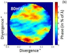
Fig. 4. (a) Optical output power of the VECSEL according to pump power and transverse beam far-field distribution (inset). (b) Far-field beam phase map at 80 mW of optical power.
