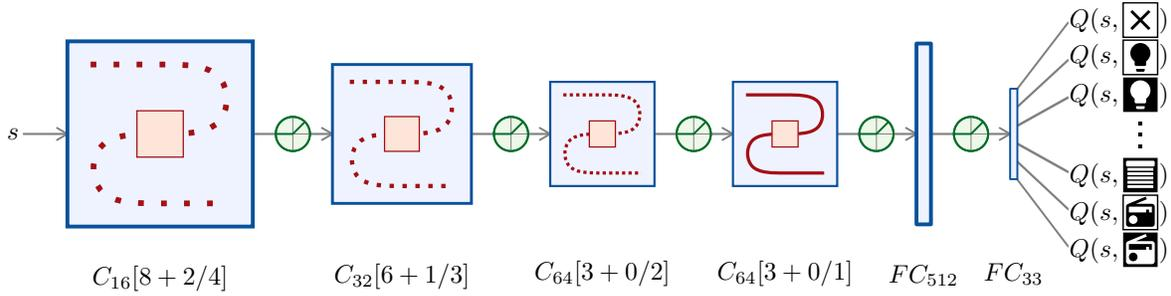
Fig. 3. Architecture of the  $Q$ -network.  $s$  is the input state (image) and  $Q(s, x)$  is the  $Q$ -value for action  $x$  given state  $s$ .  $C_n[f + p/k]$  denotes a convolution layer (using  $n$  filters of size  $f$ , with a padding of  $p$ , and using a stride of  $k$ ) and  $FC_n$  a fully connected linear layer (of width  $n$ ).
