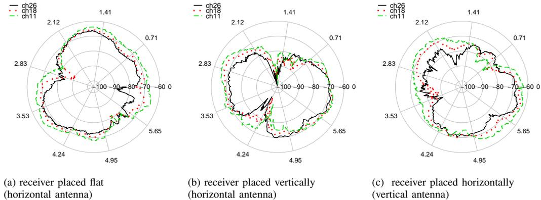
Figure 3: Reception patterns for an 802.15.4 device
