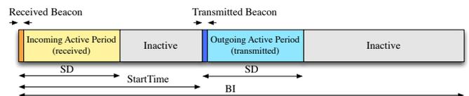
Figure 2: *Incoming* and *Outgoing* superframe structure in IEEE 802.15.4
