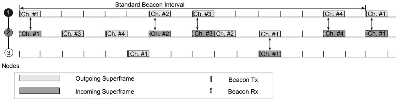
Figure 6: Principle of MRR. During the standard beacon interval delimited by two beacons on the same channel (Channel #1), a node sends additional beacons on different channels (Channels #2, #3, #4) to take advantage of channel diversity. The beaconing slots are delimited by the black vertical lines.
