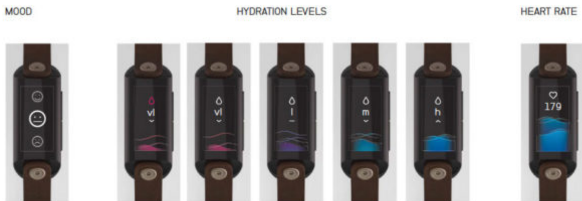
Figure 62: Wristband features to communicate mood, hydration levels, heart rate
