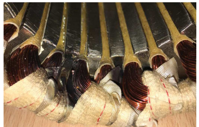
Figure 15. Stator n°1 failure at 100 mbars
