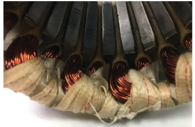
Figure 12. Stator 1: IRT Saint Exupéry typical HVDC stator
