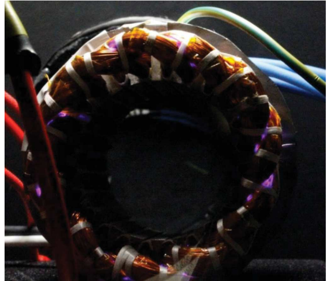
Figure 1. Partial discharge at 100mbars between phase under AC 5kHz and opening time 30s [6]
