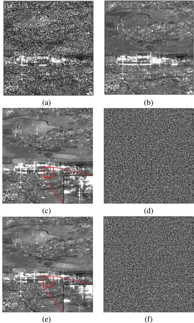
**Fig. 3:** (a)noisy Sentinel-1 data, (b)arithmetic mean image, (c)RABASAR denoised results with AM, (d)ratio between noisy data and result in (c), (e)RABASAR denoised results with BWAM, (f)ratio between noisy data and result in (e).
