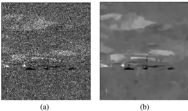
**Fig. 2:** Sentinel-1 image over Paris area. (a)ratio image, (b)MuLoG-BM3D denoised result. Appearing (dark areas in (b)) and disappearing buildings are located in the middle of the image.
