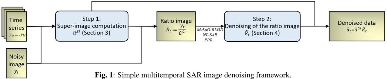
Fig. 1: Simple multitemporal SAR image denoising framework.
