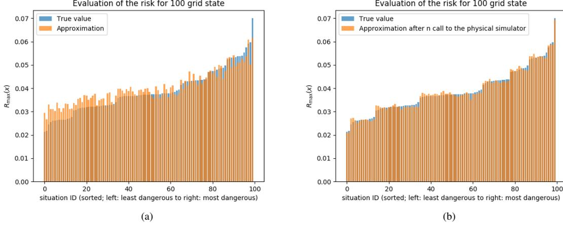
Fig. 1: **Histogram representing the total risk**, in orange is the empirical risk  $\hat{R}_{\max}$  defined in section IV. In blue is the true total risk  $R_{\max}$  for the 100 situations of the test set (a) when relying solely on machine learning (see section V-A) and (b) on allowing  $n = 186$  calls to the physical simulator (see section V-B).
