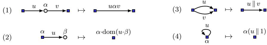
■ **Figure 3** Rewriting system for term-labeled graphs. The square vertices may have additional incident edges. The circular vertices (i.e., those that are removed) must be distinct from input and output and may not have other incident edges.
