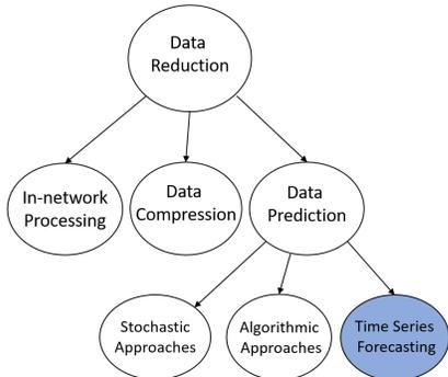
Figure 1: Categorization of energy saving in sensor networks
