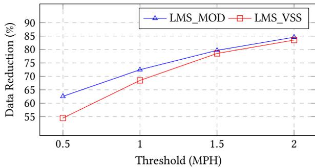
Figure 6: Data reduction for Average Wind Speed
