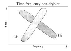
Fig. 2. TF nondisjoint condition:  $\Omega_1 \cap \Omega_2 \neq \emptyset$
