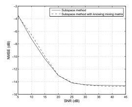
Fig. 7. Comparison, for the subspace-based TF-UBSS algorithm using STFT, when the mixing matrix  ${\bf A}$  is known or unknown: NMSE of the source estimates.
