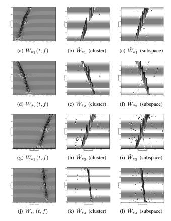
Fig. 10. Simulated example (viewed in TF domain) for the subspace-based TF-UBSS algorithm with STFT in the case of 4 LFM sources and 3 sensors. From left to right, the figures respectively represent the original source TF signatures, the estimated source TF signatures using the cluster-based algorithm, and the estimated source TF signatures using the subspace-based algorithm.
