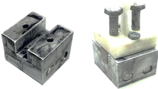
Fig. 3. Pictures of molds used in composites manufacturing.
