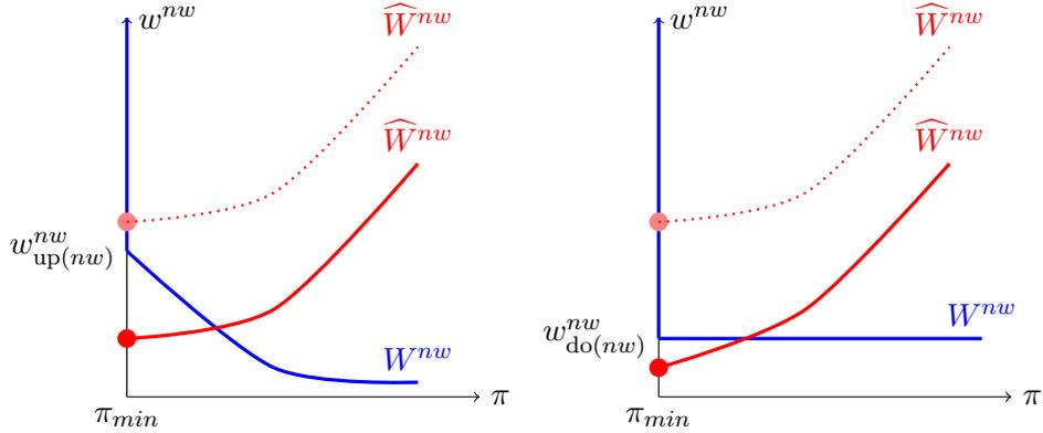
Figure 2: The values of  $W^{nw}$  and  $\widehat{W}^{nw}$  versus capillary pressure  $\pi$  in non-degenerate (left) and degenerate (right) two phase cases.
