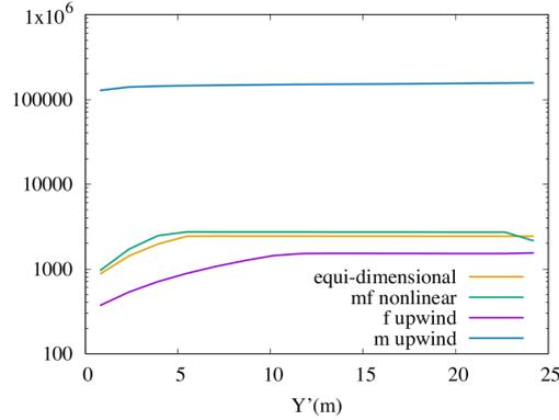
Figure 8: Capillary pressure in Pa at final time in the bottom fracture  $\Gamma_4$  as a function of  $y'$  for the equi-dimensional model (average in the fracture width), the  $mf$  nonlinear model, the  $mf$  linear  $f$  upwind model and the  $mf$  linear  $m$  upwind model.
