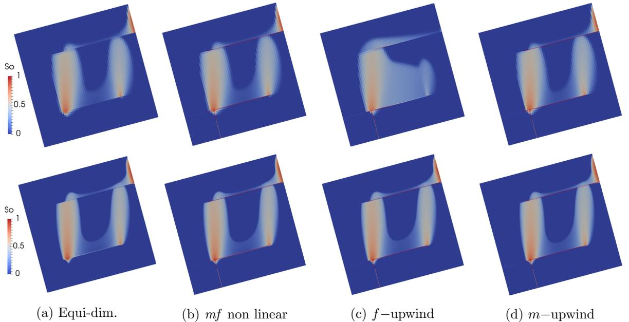
Figure 6: From left to right: oil saturation at final time for the equi-dimensional and hybrid-dimensional models. Top row: Cartesian mesh of size  $68 \times 72$  for the equi-dimensional model and of size  $64 \times 64$  for the hybrid-dimensional models. Bottom row: Cartesian mesh of size  $260 \times 264$  for the equi-dimensional model and of size  $256 \times 256$  for the hybrid-dimensional models.
