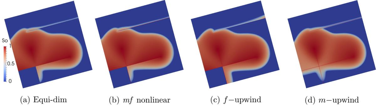
Figure 9: From left to right: oil saturation at final time computed by the equi-dimensional and hybrid-dimensional models for the viscous dominant test case with overpressure of  $2 \cdot 10^6$  Pa
