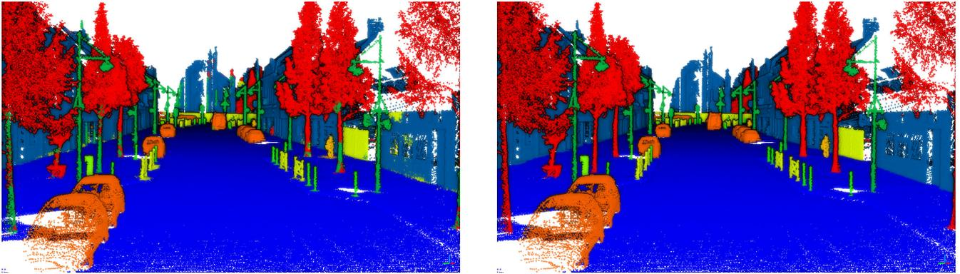
Fig. 4. Example of classified point cloud on Paris-Lille-3D dataset. Left: classified with MS3\_DVS, right: ground truth (blue: ground, cerulean blue: buildings, dark green: poles, green: bollards, light green: trash cans, yellow: barriers, dark yellow: pedestrians, orange: cars, red: natural).
