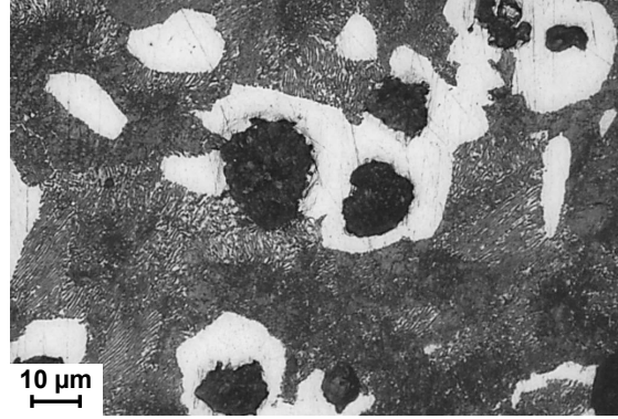
Figure 3: Optical micrograph of the ASTM A536 100-70-03 iron in its original state (etched with saturated nitric acid).
