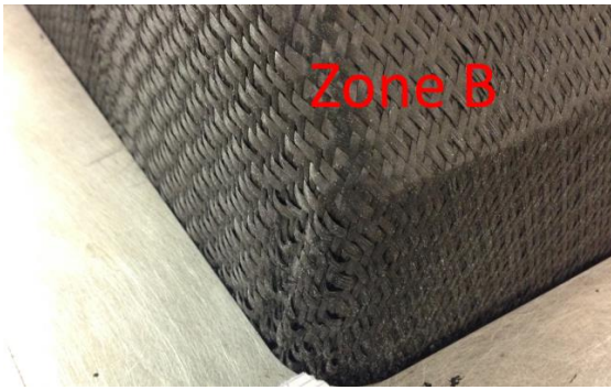
Figure 5 : Quality preform with pressure increasing, case of monolayer oriented at 30°
