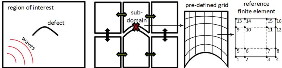
**Figure 1.** From left to right: a 2D surface with a parametric defect; the same surface divided into six sub-domains; a deformed pre-defined grid; a finite reference element and 16 DoFs located by a quadrature rule of order 3.
