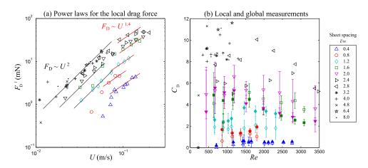
FIG. 4. (a) Log-log representation of the same data as Figure 3(b). The black continuous line shows the trend  $F_D \propto \overline{U}^2$  for small  $\overline{U}$  and the red dashed line  $F_D \propto \overline{U}^{2+V}$  for large  $\overline{U}$ . (b) Non-dimensional comparison with the *global* profile drag measured from the pressure loss across the channel (closed symbols). Open symbols represent the *local* data from individual sheet deflection measurements.
