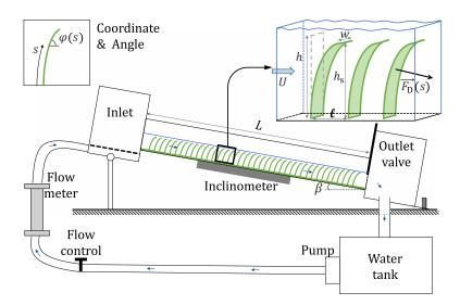
FIG. 1. The experimental setup. The open channel has an adjustable water flow rate Q and inclination angle  $\beta$ . An array of PVC sheets representing an aquatic canopy is fixed all along the channel. The outlet valve is set to adjust the water height  $h_w$ .
