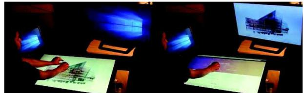
**Figure 5:** A Translation + Spread gesture sends the tabletop content (left) to a secondary display (right).
