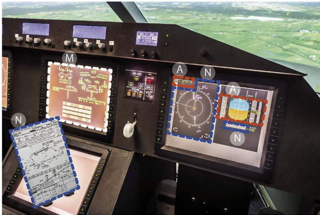
Fig. 2. Cockpit interior from participant's point of view showing the definition of AoI sets: Aviate (A), navigate (N), and system management (M).
