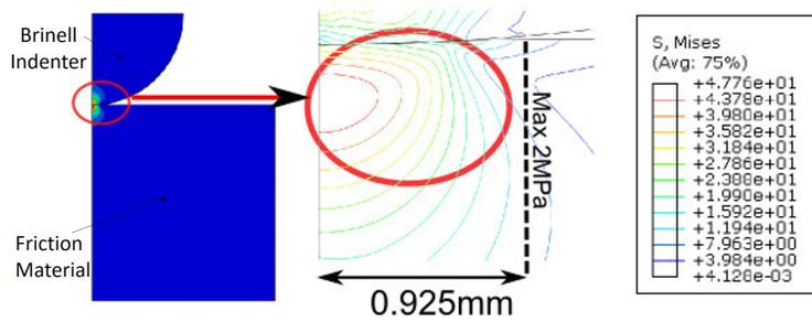
Figure 2: 2D axisymmetric model of indentation tests for definition of the mapping of the friction pad
