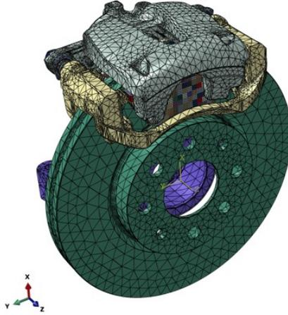
Figure 9: Finite element model of the automotive brake corner.
