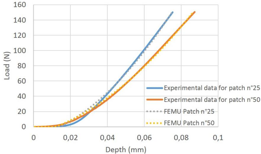
Figure 4: Inverse identification with FEMU method on patch  $n^{\circ}25$  and  $n^{\circ}50$
