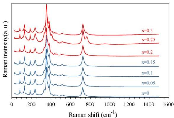
Fig. 3. Raman spectra for  $\text{La}_{3-x}\text{Sr}_x\text{CuTaO}_{7-x/2}$ ,  $x = 0, 0.05, 0.1, 0.15, 0.20, 0.25, 0.30$ .
