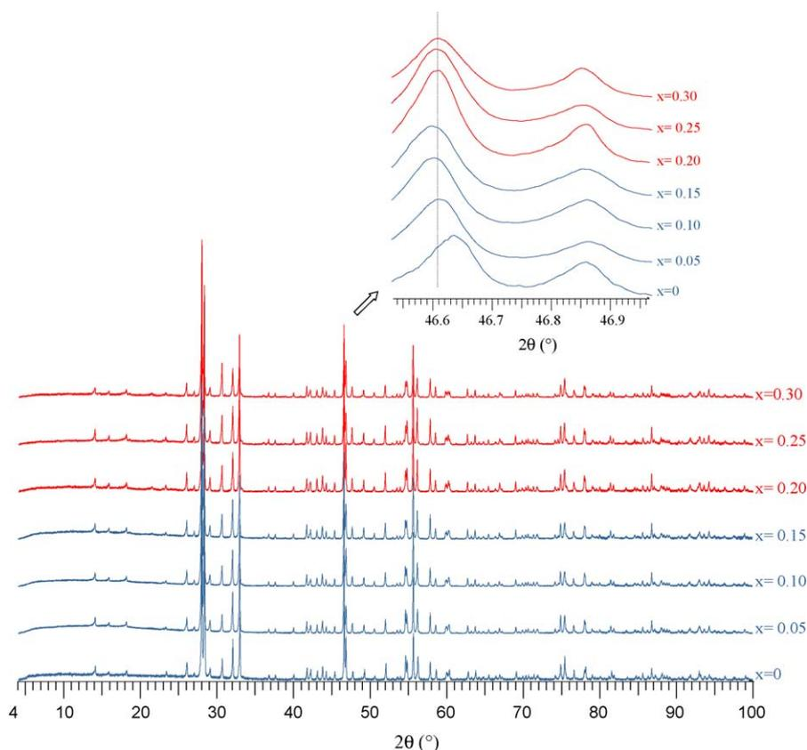
Fig. 2. X-ray diffractograms corresponding to  $\text{La}_{3-x}\text{Sr}_x\text{CuTaO}_{7-x/2}$ ,  $x = 0, 0.05, 0.10, 0.15, 0.20, 0.25, 0.30$ .
