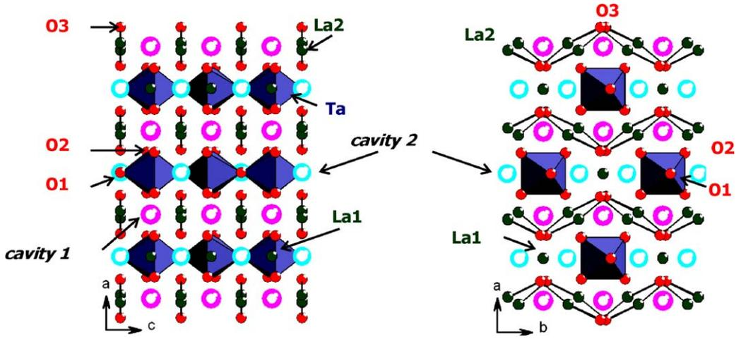
Fig. 1.  $\text{La}_3\text{TaO}_7$  crystalline structure in  $\text{Cmcm}$  space group with evidence of two cavities.
